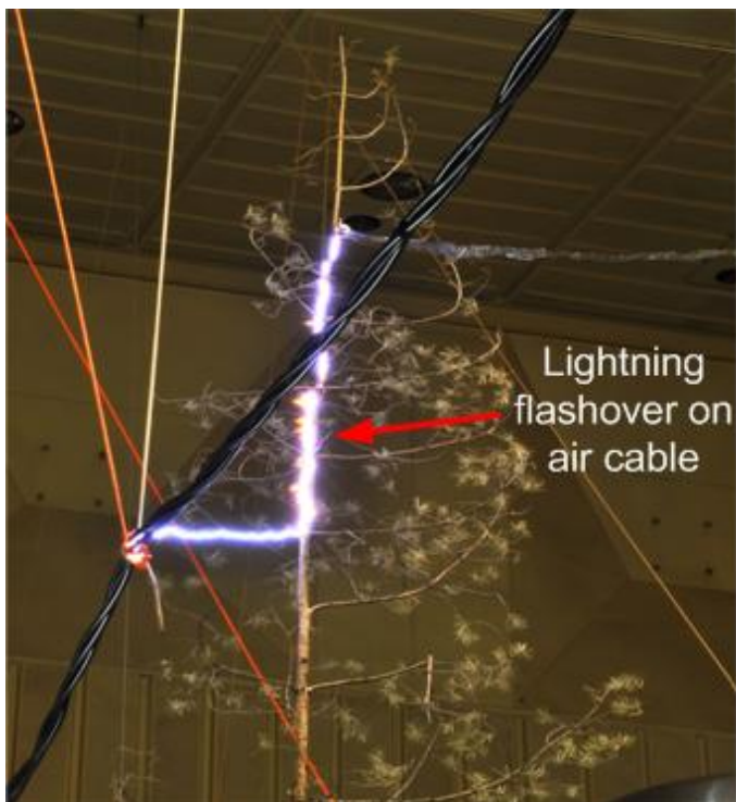
Figure 3.4. Lightning flashover to air cable from the lightning-struck tree
