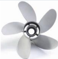
Propeller for racing boats as scaled model for flow measurements
