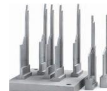
Mould inserts with integrated, surface conformal cooling channels. Photo with kind permission of Gardena AG
