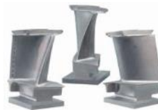
Turbine blade of latest generation with internal conformal cooling channels to improve performance of jet engines
